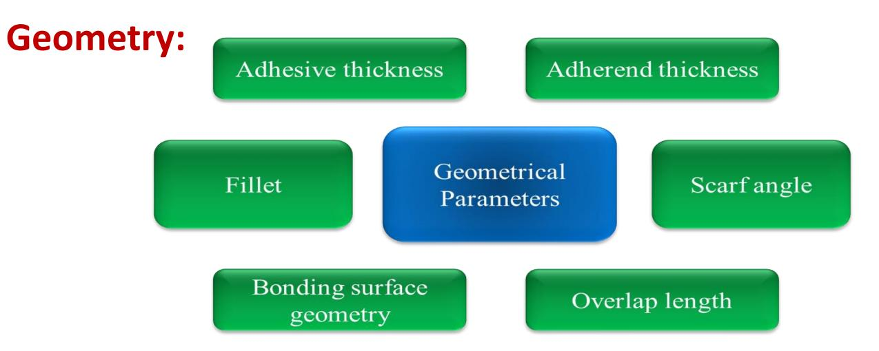
Increasing overlap length generally reduces the fatigue strength in bonded joints for the same fatigue load ratio. Strategies like fillet creation, groove patterns, and sinusoidal/zig-zag geometries on overlap surfaces enhance fatigue strength.
